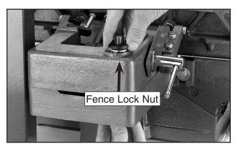
**Figure 3.** Removing the fence lock nut so the sliding surfaces can be cleaned.
